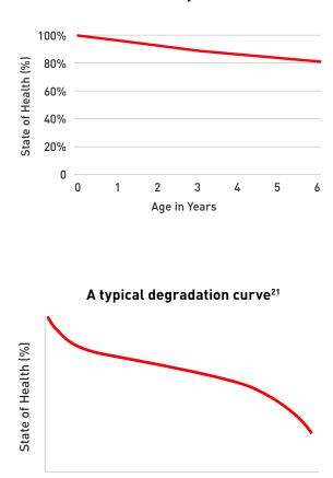
Average battery deterioration as shown by Geotab<sup>21</sup>
